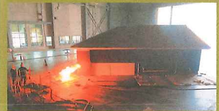
Figure 2a Experiments conducted at the IBHS Research Center to study the effectiveness of creating a noncombustible space around buildings.
